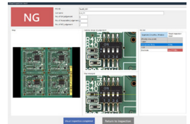
You can specify the approximate location on the map image and specify the detailed location by zooming in on the map. You can also refer to the image at the time of judgment.
