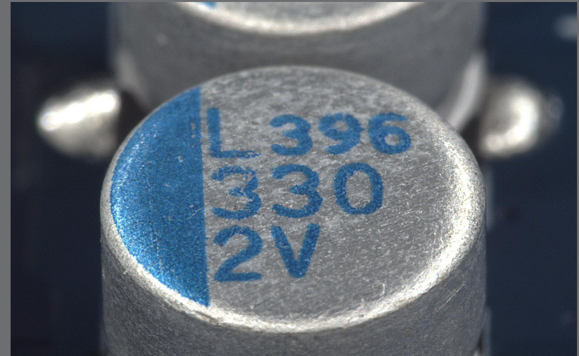
Thanks to the Z-axis, characters on the upper surface of high parts can be clearly confirmed without blurring. Images with a deep depth of field make it easy to detect human errors such as wrong parts.
